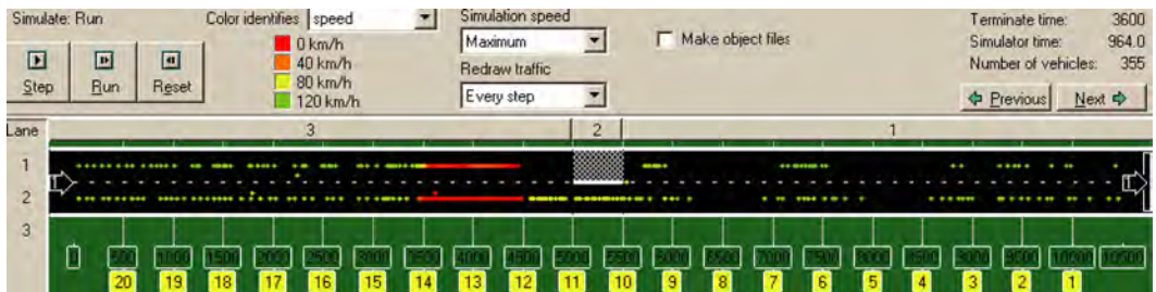
FIGURE 10. Screenshot of freeway stretch with a temporary bottleneck (e.g., an incident) coded in microsimulation model FOSIM (Vermijs and Schuurman [55]).
